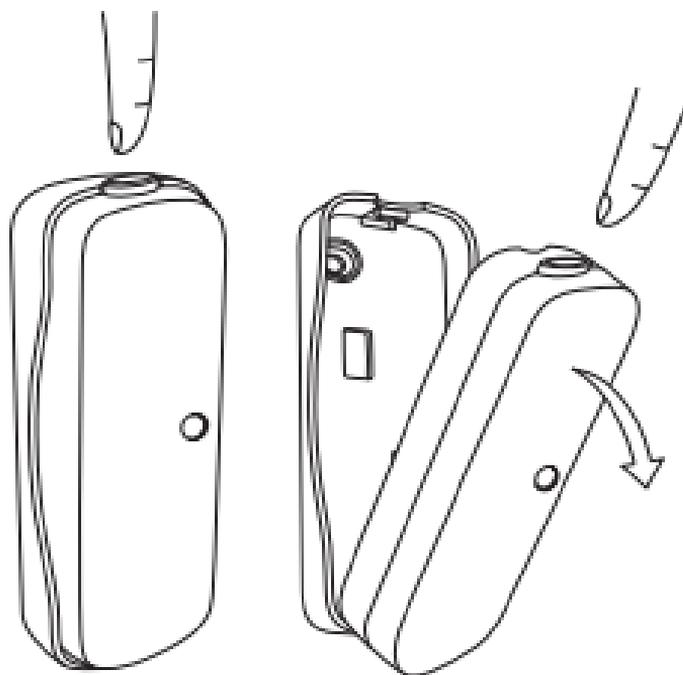
8.2 Insert the CR2 with the negative end first depressing the battery spring.
